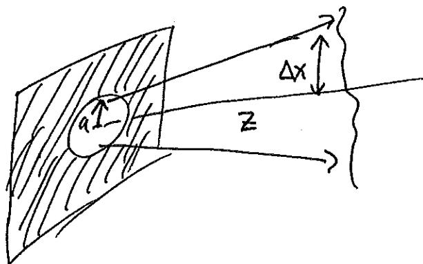
$$\delta(\Delta x, \Delta y) = e^{-i\frac{\pi}{2}} \left[ \frac{J_1\left(\frac{2\pi a}{\lambda z} \sqrt{\Delta x^2 + \Delta y^2}\right)}{\frac{2\pi a}{\lambda z} \sqrt{(\Delta x)^2 + (\Delta y)^2}} \right]$$
