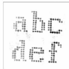
Figure 4 The specimen image as reconstructed from the diffraction pattern of Fig. 2.
