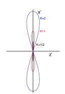
$$\begin{array}{rcl} \textbf{\textit{v}}_{\textbf{\textit{z}}} & = & c \left( 1 - \frac{1 + K^2/2}{2\gamma^2} - \frac{K^2}{4\gamma^2} \cos 2\textbf{\textit{k}}_{\textbf{\textit{u}}}\textbf{\textit{z}} \right) \\ \textbf{\textit{v}}_{\textbf{\textit{x}}} & = & \frac{cK}{\gamma} \sin \textbf{\textit{k}}_{\textbf{\textit{u}}}\textbf{\textit{z}} \end{array}$$
