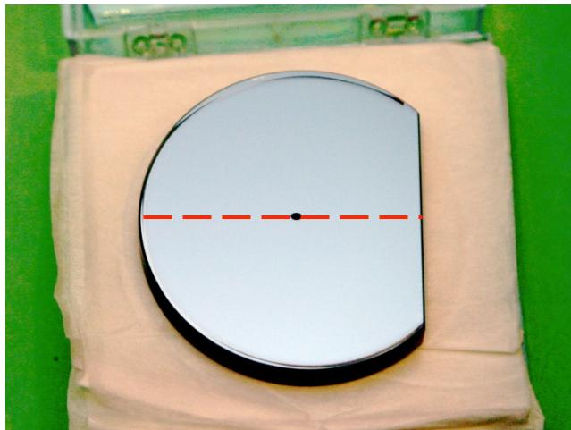
Multilayer coated mirror with high lateral gradient. The red line indicates the line scan direction.
