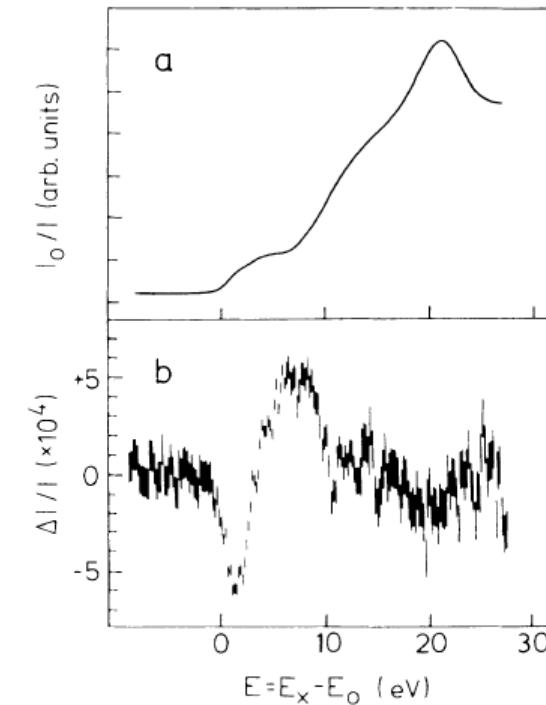
FIG. 1. (a) Absorption  $I_0/I$  of x rays as function of the energy  $E$  above the  $K$  edge of iron and (b) the difference of the transmission  $\Delta I/I$  of x rays circularly polarized in and opposite to the direction of the spin of the magnetized  $d$  electrons.
