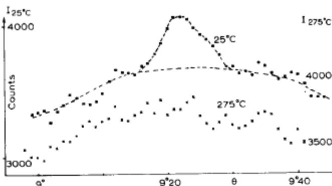
Fig. 1. Intensity  $I_f(\theta)$  near the  $(\frac{1}{2} \frac{1}{2} \frac{1}{2})$  position at  $t = 25^\circ \text{C}$  and  $275^\circ \text{C}$  in counts/225 min. The hump which cover the interval could be due to some impurity.
