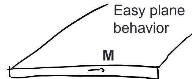
$K_{1,\text{eff}} < 0$  for  $t > 2 \text{ nm}$
