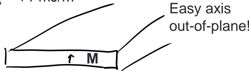
→  $K_{1,\text{eff}} > 0$  for  $t < 2 \text{ nm}$  !!!
