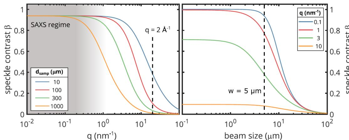
Reduced speckle contrast at large  $q$  (molecular length scales) because of longitudinal coherence length  $\rightarrow$  path length differences
