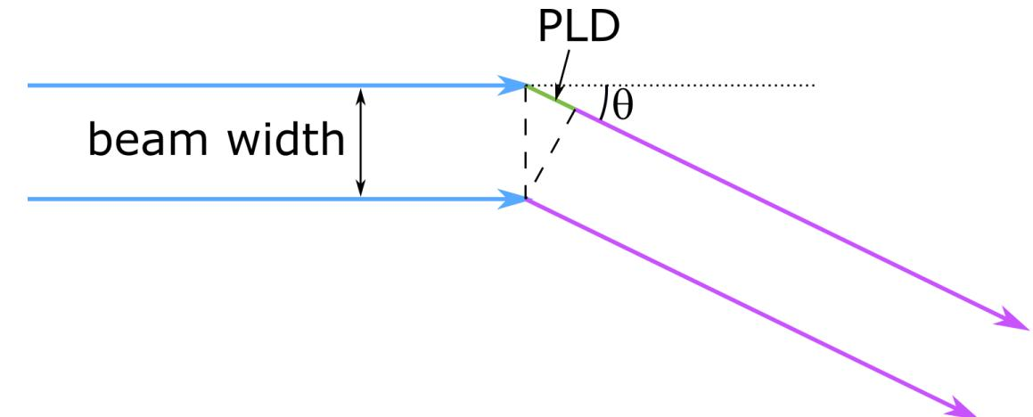
$$\text{SAXS: } \theta \approx 0.1^\circ \rightarrow \text{PLD} < 0.02 \mu\text{m}$$
