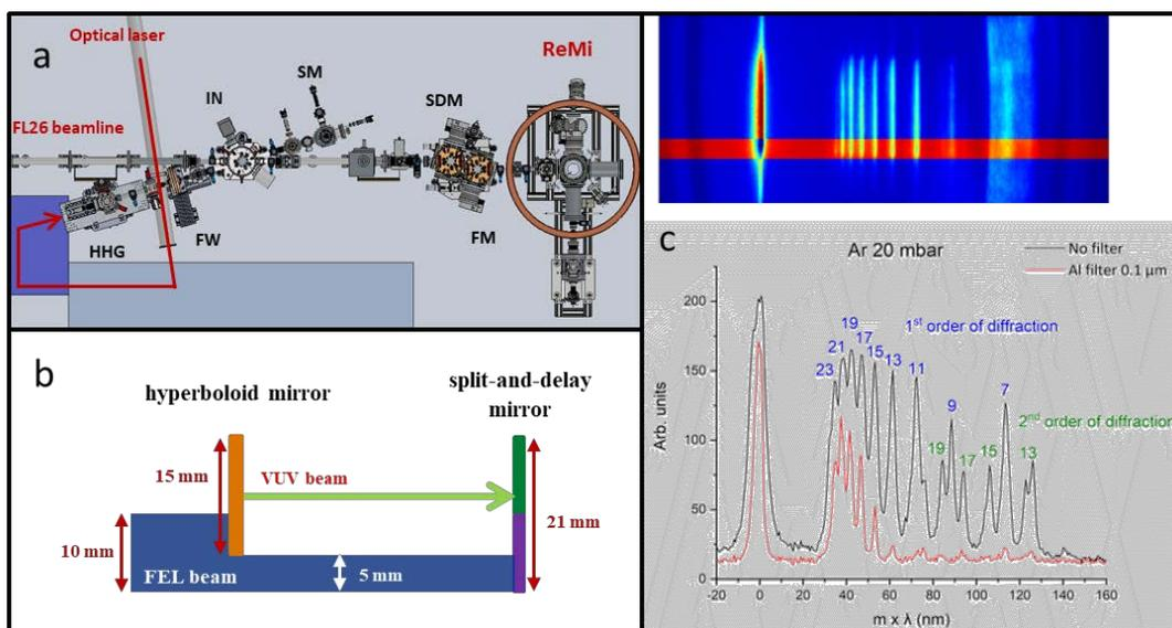
**Fig. 1 a)** HHG beamline incorporated in the FL26 beamline. HHG: HHG chamber, FW: filter wheel, IN: in-coupling chamber, SM: spectrometer, SDM: split-and-delay mirror, FM: focusing ellipsoidal mirror **b)** the lower part of the FEL beam is centered in the lower half of the split mirror **c)** harmonics spectrum on the phosphor screen, calibrated with respect to  $m \times \lambda$  ( $m$ : order of diffraction,  $\lambda$ : wavelength)
