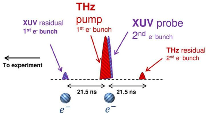
**Figure 1:** THz doubler timing scheme: 1st electron bunch generates “residual” XUV pulse and THz pump pulse, while 2nd generates XUV probe (temporally overlapped at the experiment with THz pump) and “residual” THz pulse. Residual pulses are not used in pump-probe experiment.
