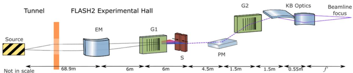
**Figure 4:** Schematic of the Time Delay Compensating Monochromator beamline FL23 (not to scale).
