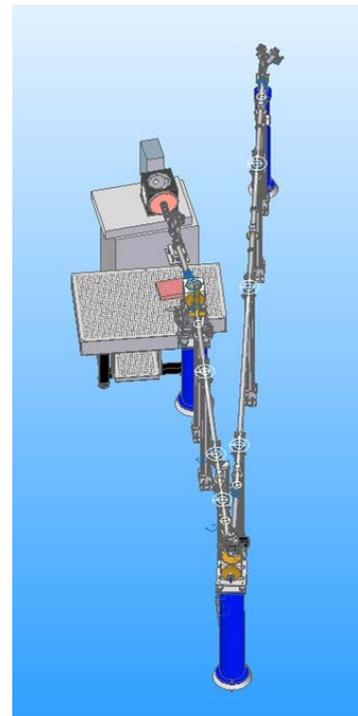
**Figure 3:** End of beamline FL21 with two branches: pulse length diagnostics (left) and open port for exploratory setups (right).
