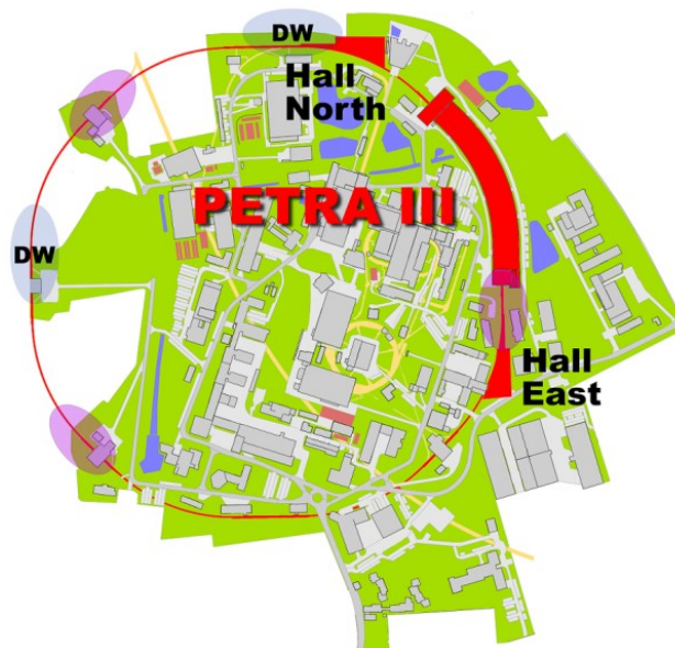
Figure 1.1: View of the PETRA III storage ring (red line). The present experimental hall is shown together with the planned additional experimental halls in the North and East.
