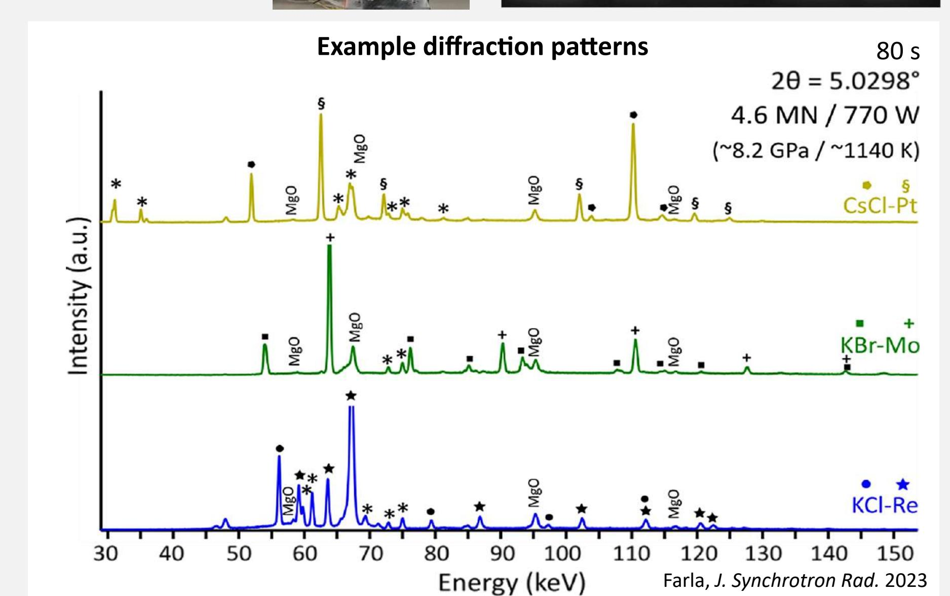
Multiple materials can be accommodated in the same cell assembly at similar high pressure-temperature (HPHT) conditions for complete structural characterisation by ED-XRD over large ranges of HPHT.
