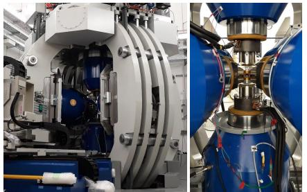
2. Purchase of new PE press: moderate pressures (15 GPa) on liquid/solid samples.
