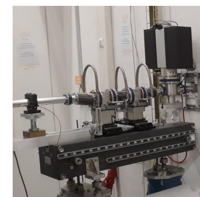
Incident slits before LVP in EH2 (P61B) 10 mm slit blades [Densimet, (Ni,Fe)_{0.02}W_{0.98} ]
