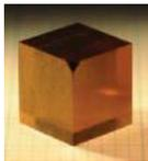
Anvil truncation is typically 1.5 mm for UHP experiments in the LVP using Kawai-8 cubic anvils set ups. Sample size is up to 0.5 mm.
