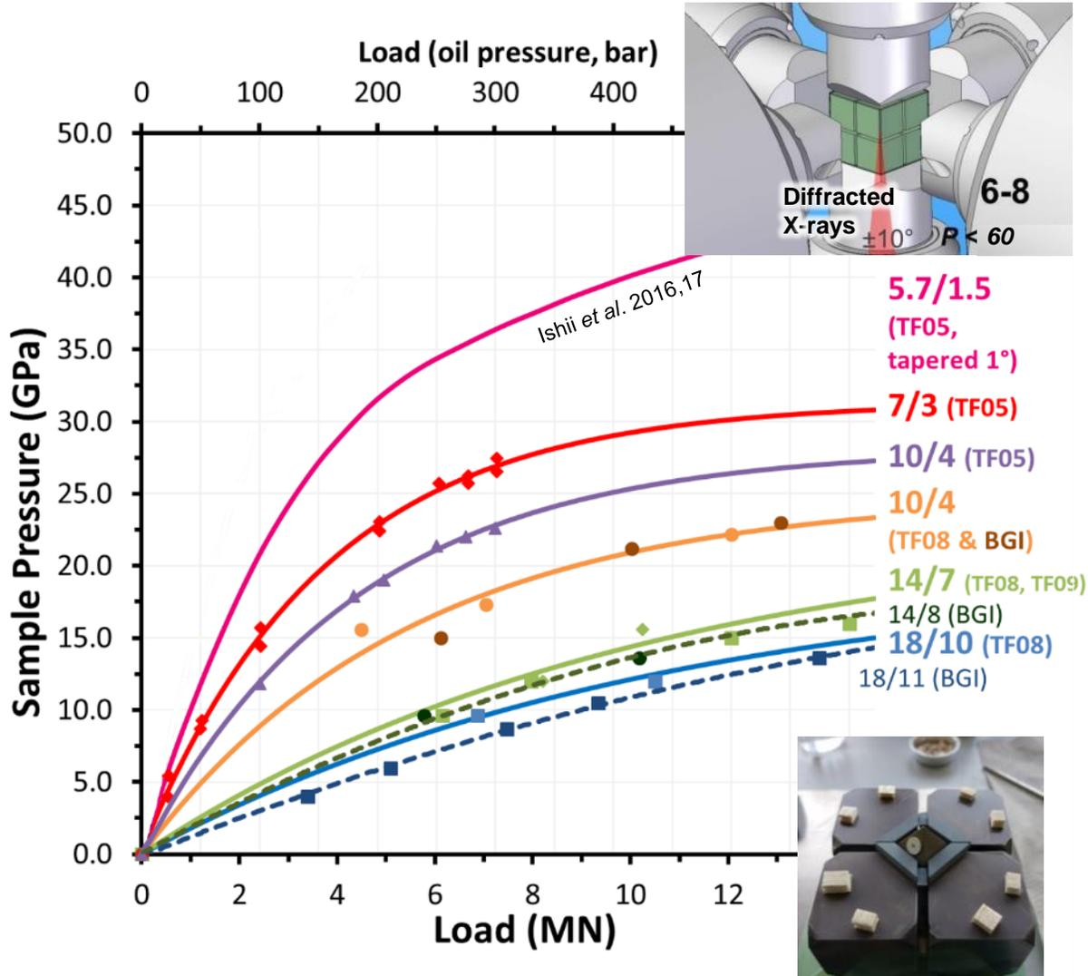
**Anisotropic compression:** for *in situ* rock deformation studies using MA6-6 set ups (max. 15 GPa / 2000 K)
