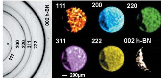
2D XRD pattern and 2D reconstructed slices from *d*-spacing/ $2\theta$  of different reflections ( $C_{60}$  polymerization under pressure).
