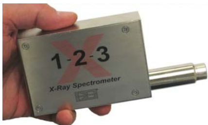
Figure 2a. The X-123 configuration, which includes the detector, preamplifier, digital processor, and power supplies all in one box.
