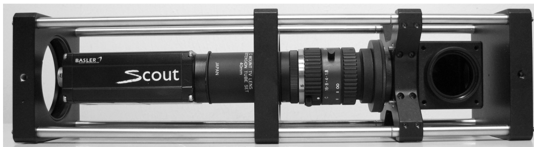
Figure 3: X-ray camera with a Basler Scout SCA640-74gm Gigabit Ethernet camera.
