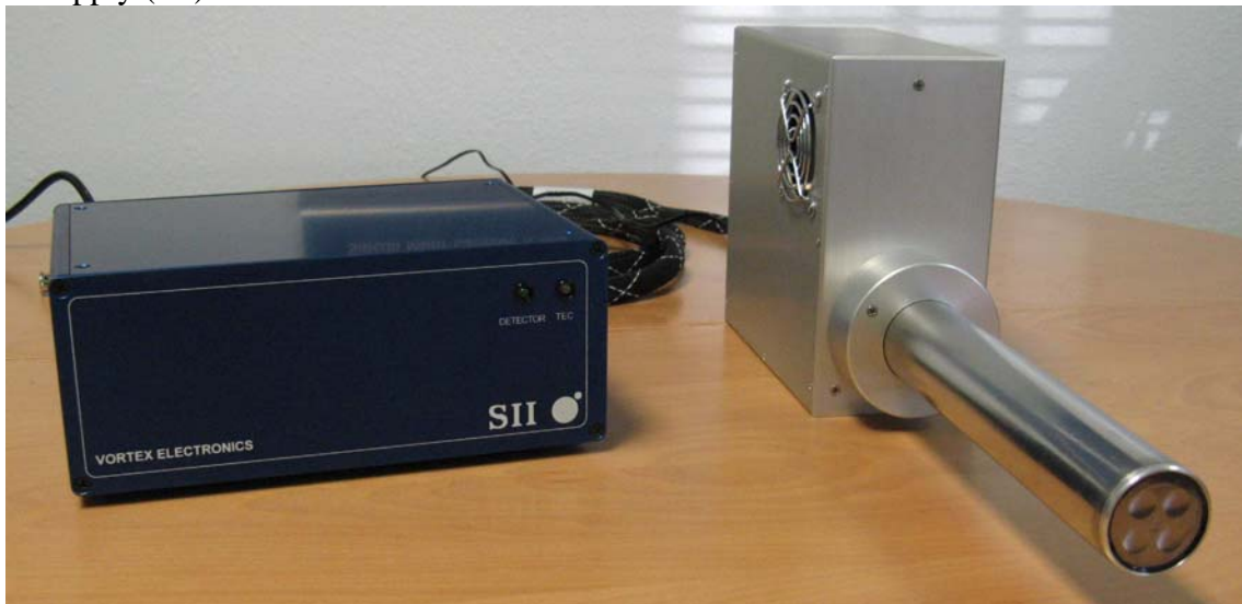
Figure 1. The Vortex-ME4 ™ multi-element detector system. Left to right: PS box, cable, SDD package.
