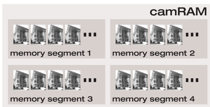
Figure 3.2: Illustration of the camera's primary image memory (camRAM). The image memory is divided into four memory segments (memory segment 1-4), which accepts the images for storage.
