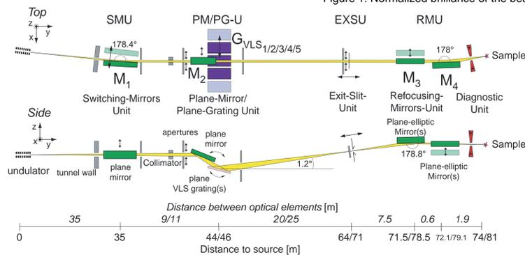
Figure 2: Optical layout of the beamline P04.
