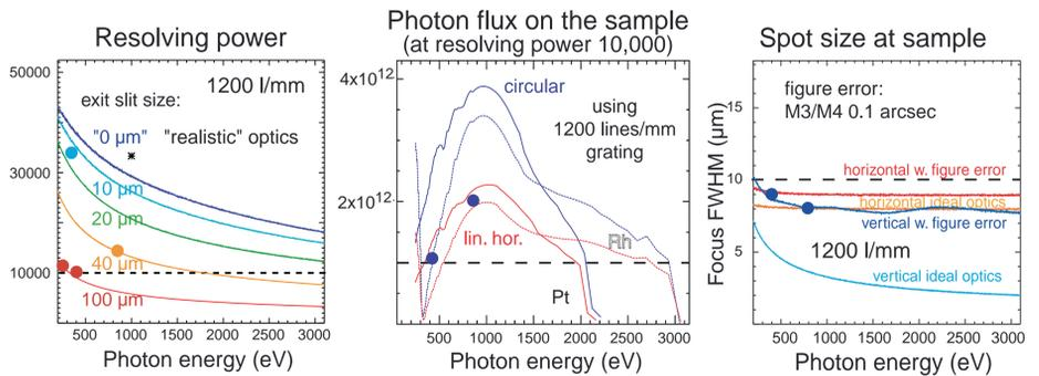
Figure 3: Performance of the beamline P04 (lines: calculated values, circles: measured values).
