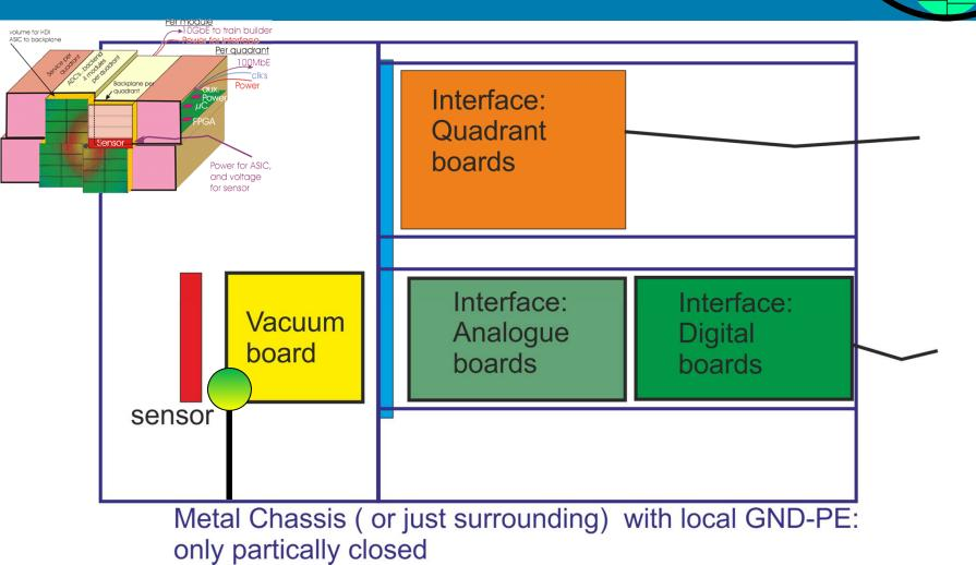
1. Choose main grounding point: At most sensitive part the detector plane
