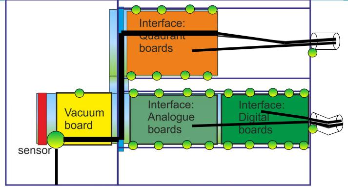
Metal Chassis (or just surrounding) with local GND-PE: only partically closed
