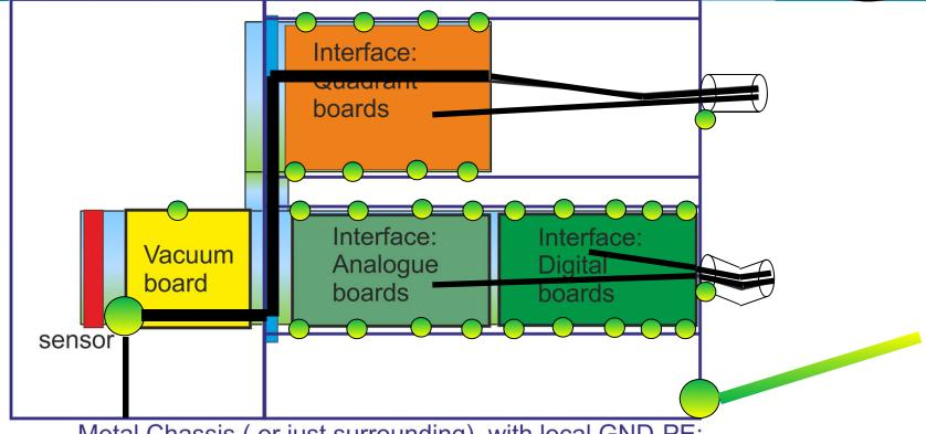
Metal Chassis (or just surrounding) with local GND-PE: only partically closed
