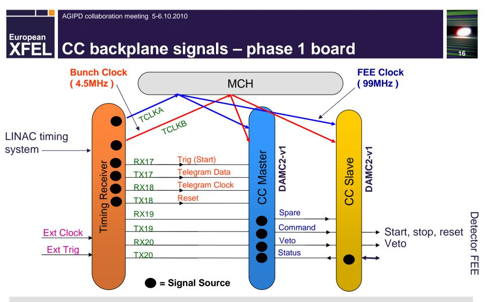
Phase 1 = TR board clock distribution + MCH jitter ~100ps phase 2 = DAMC2-v2 clock distribution + MCH jitter ~few ps
