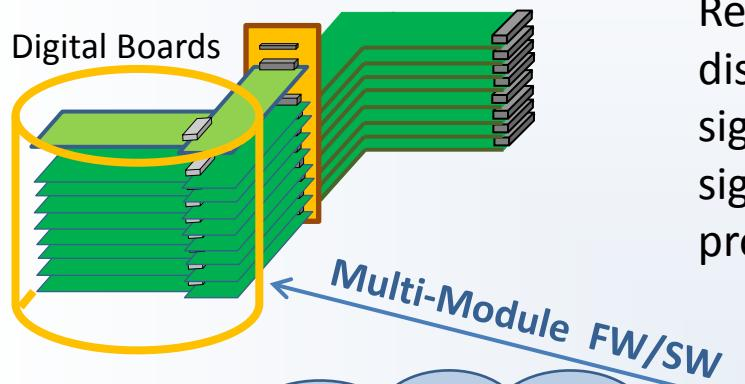
Readout sequence , triggering, C&C information,.. distributed by two Control modules via dedicated signal lines to (8+8)Readout modules. According these signals Readout modules execute all proper data processing and send these data to Back-End.
