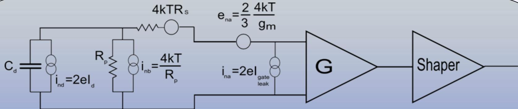
$$Q_n^2 = \frac{\exp(2)}{8} \left[ \left( 2eI_d + \frac{4kT}{R_p} + i_{na}^2 \right) \tau + \left( 4kTR_s + e_{na}^2 \right) \frac{C^2}{\tau} + 4A_f C^2 \right]$$
