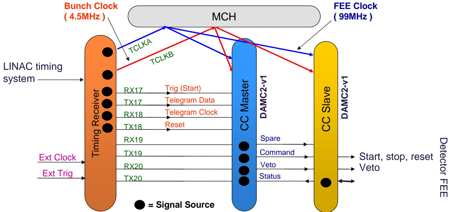
Phase 1 = TR board clock distribution + MCH jitter ~100ps
