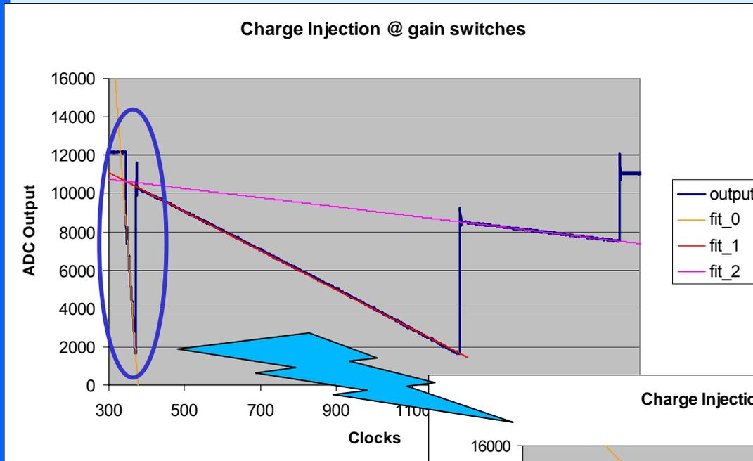
Charge Injection @ first switch is significant and have to be calibrated
