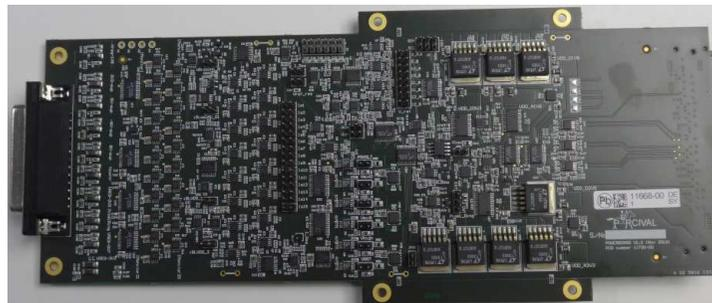
PowerBoard for sensor supply & biasing
