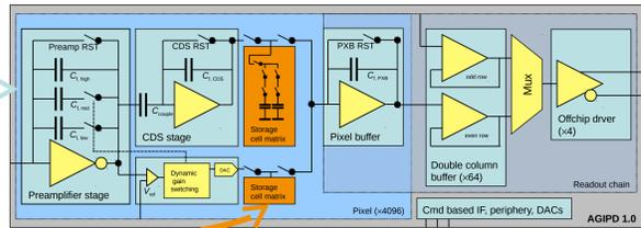
AGIPD ASIC: Pixel layout (left) and block diagram showing the analogue readout chain (top)
