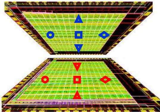
Different pixels/samples: slightly higher variations. However, outputs from memory cells in the Top/Bottom tier of the same pixel remain similar.
