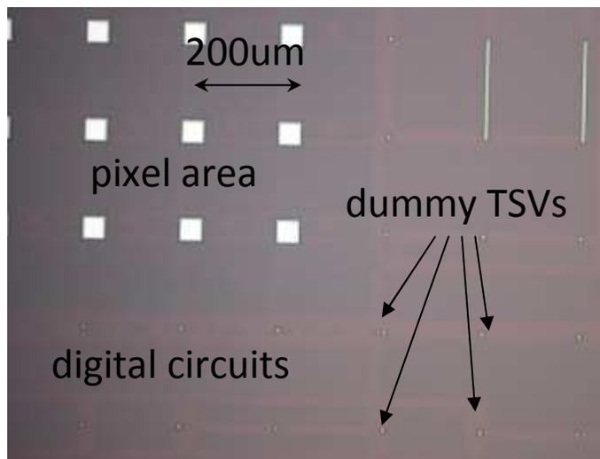
10x test structure for TSV evaluation: daisy chain of 64 TSVs, by connected M1/backM.
