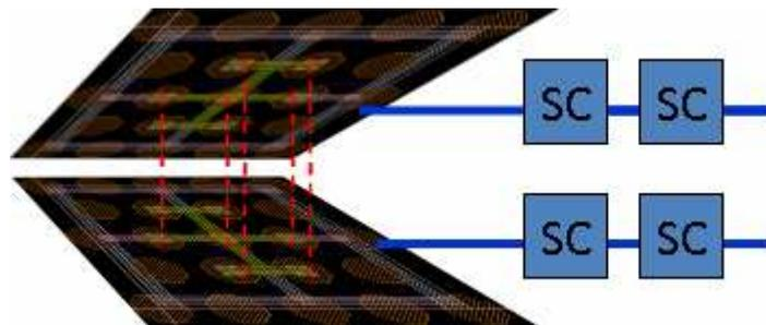
tier-to-tier contact redundancy was suggested by 2009 MPW experience, to counter eventual tier misalignment
