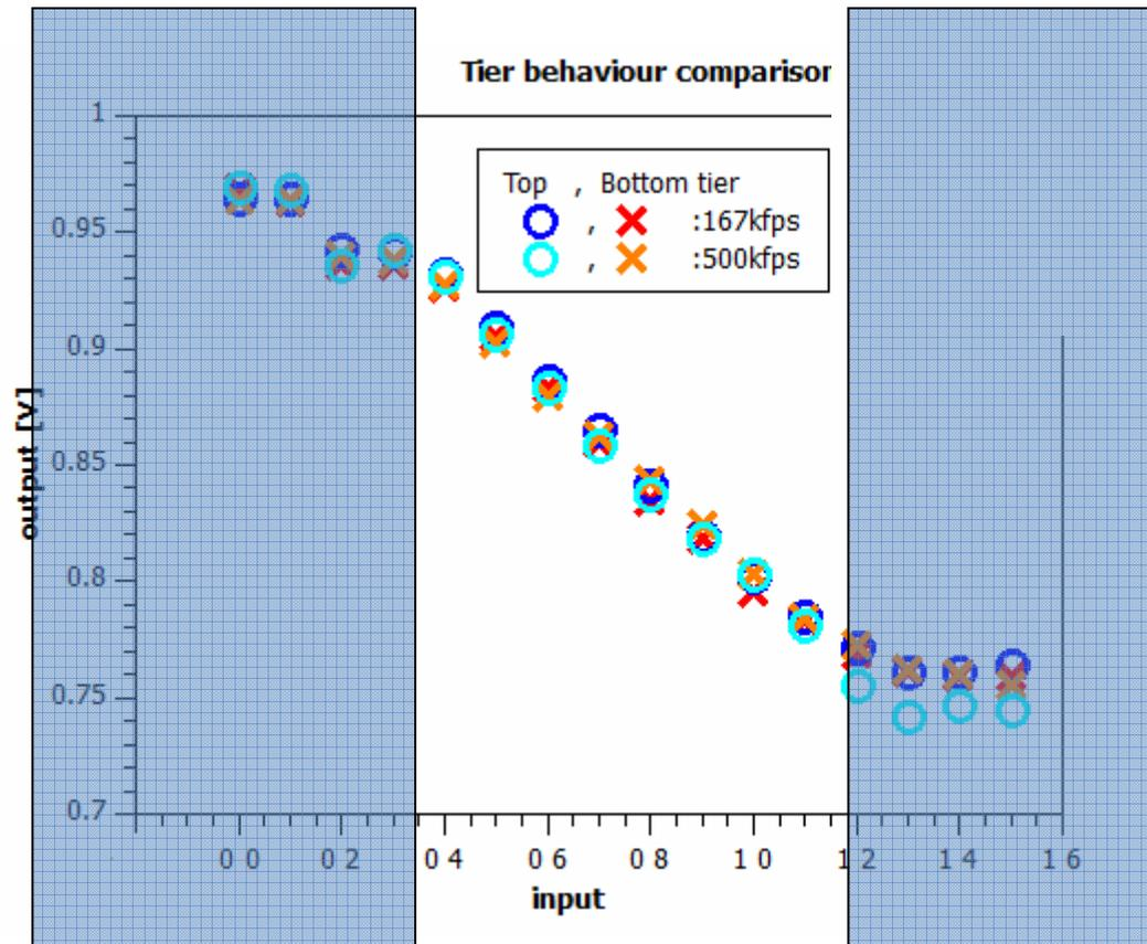
expected operation region of the circuit: comparable (linear) behaviour of the detector output, whether the charge is stored in/read from storage cells located on the Top tier or Bottom tier
