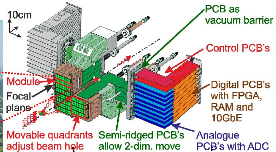
Hybrid (Si-Si) charge integration x-ray detector
