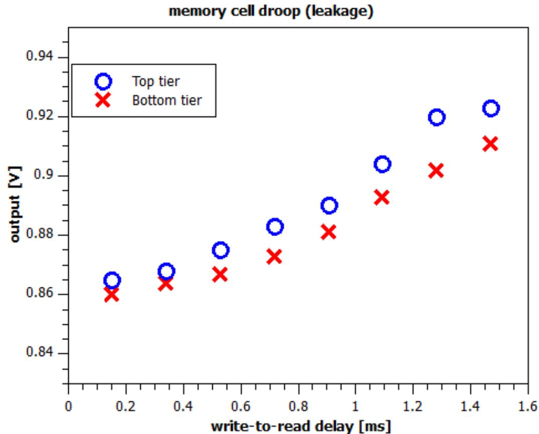
significant parasitic leakage of charge stored in memory cells
