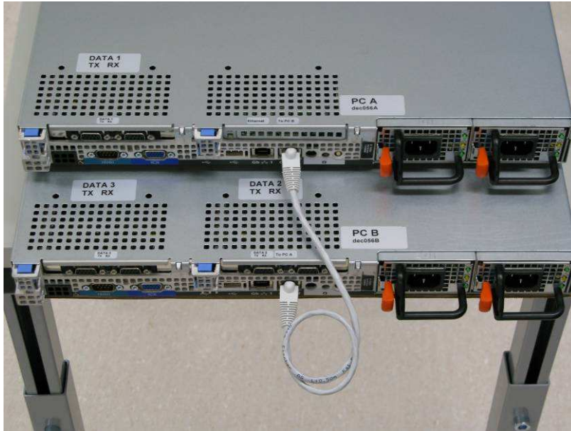
Figure 6 Detail of interconnection between PC A and PC B. (Data cables not connected for better demonstration)
