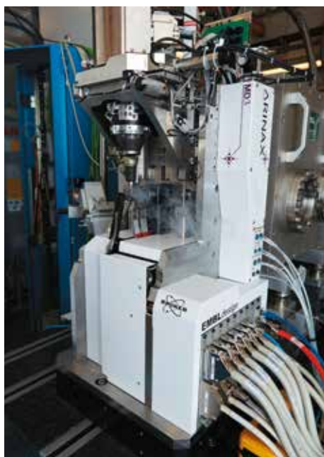
Figure 1 Crucial for the success of this experiment was the high-precision vertical MD3 microdiffractometer at the P14 beamline – developed by scientists and engineers at EMBL Hamburg and EMBL Grenoble – and the micrometre sized high-flux X-ray beam at the PETRA III storage ring.
