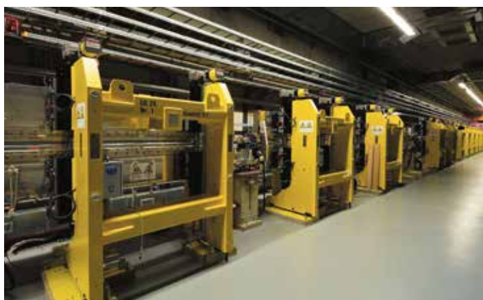
The 30 m long undulator in the FLASH2 FEL line, consisting of 12 segments, which produces the FEL radiation.
