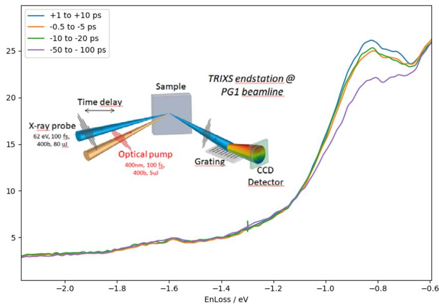
**Figure 2:** Co M-edge RIXS spectrum as function of (binned) pump-probe delays measured with the TRIXS endstation at PG1. Positive delay means unpumped, i.e. optical laser arrives after FEL; negative delay means pumped (optical pump laser arrives before the FEL).
