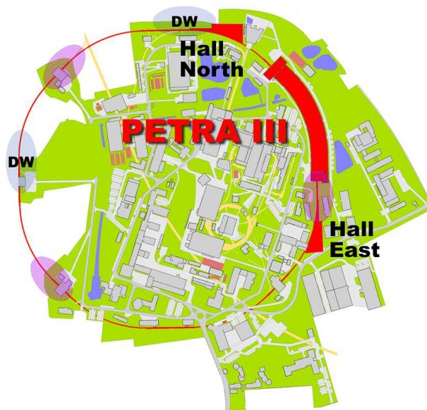
Figure 1.1: View of the PETRA III storage ring (red line). The present experimental hall is shown together with the additional experimental halls in the North and East which are currently under construction.
