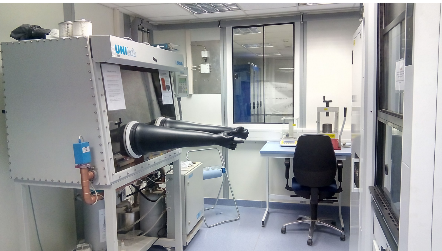
P64/65 sample preparation lab with equipped with a fume hutch, glove box, infrastructure for use of gases, sample press, analytical balance...
