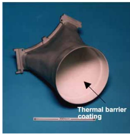
Zr K EXAFS spectra measured in Eu 2 Zr 2 O 7 nano particles, illustrating the evolution of crystallinity versus annealing temperature. Step scans, 10 min per scan, powder samples (R. Chernikov, DESY), substances like these are used as thermal barrier coatings for gas turbine transition ducts (see right picture) etc. A. P. Menushenkov et al, Moscow Engineering Physics Institute, Moscow, Russia
