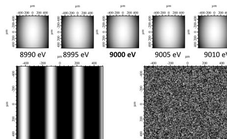
Upper row: Intensity distributions ( $I_0$ ) at different DCM-energies and constant undulator gap
