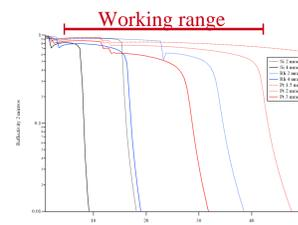
Cumulated reflectivity of two plane mirrors at varying angles of incidence. The presented reflectivities include the effect of a conservatively estimated value of 5 Å for the roughness of the mirror surface. The mirror in front of the DCM is reducing the power load on the 1<sup>st</sup> DCM crystal.
