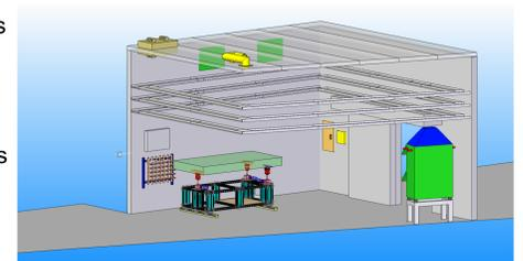
CAD drawing of the experimental hutch of beamline P65. Visible are the experimental table, and the air-conditioning system. The size of the hutch is approximately  $30 \text{ m}^2$ , the height of the ceiling  $\sim 4\text{m}$ .
