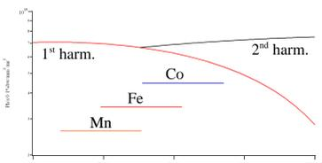
Brilliance of a 12 periods U32.0 undulator with  $K_{\text{max}} = 2.6$  (magnetic gap 10.05 mm), overlap between 1<sup>st</sup> and 3<sup>rd</sup> harmonic and scan ranges of Mn, Fe and Co standard EXAFS scans.
