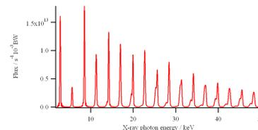
Flux through an aperture ( $1^*2 \text{ mm}^2$ ) in 60 m distance from a 12 periods U32.0 undulator with K tuned to 2.384 (5<sup>th</sup> harm. at 20000 eV)
