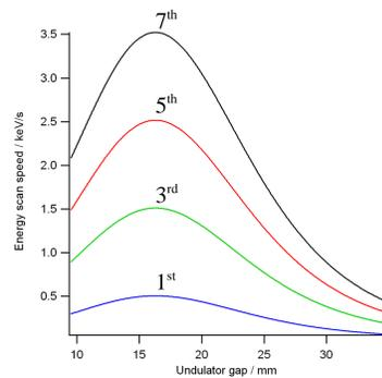
Maximum energy scan speed for U32.0 undulator
