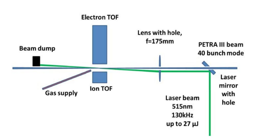
Schematic of the XUV-pump – laser probe experiment. The laser system is synchronized to the storage ring with a residual jitter of ~15ps. Every 40<sup>th</sup> bunch can be pumped at ~130kHz repetition rate.
