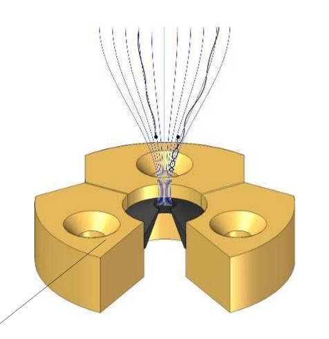
Assembly of three magnets and pole cap generating the magnetic field. The bottle neck shape turns electron trajectories upwards to the detector while the kinetic energy is conserved.
