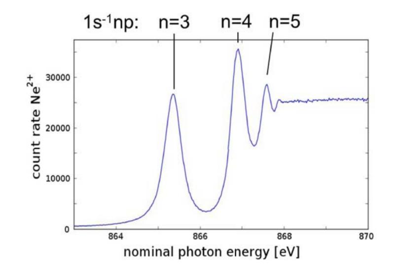
Ne<sup>2+</sup> ion yield at the Ne1s ionization threshold showing the first resonant rydberg states of the 1s-np-excitation.
