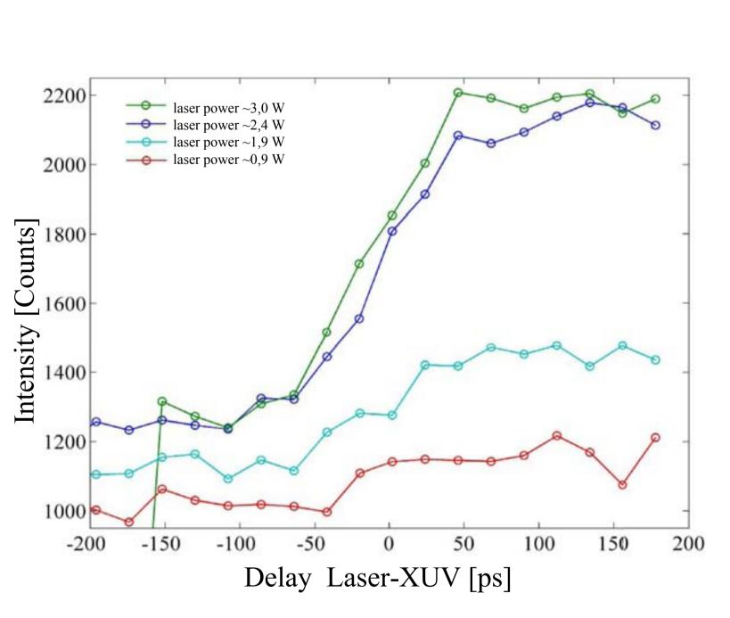
Ion yield of Ne<sup>2+</sup> in coincidence with slow electrons vs. laser delay and laser power. The rise time of the signal corresponds to the pulse duration of the X-ray pulses of ~100 ps.
