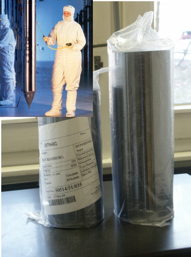
Silicon single crystal ingots 4inch dia., length 25cm-30cm
