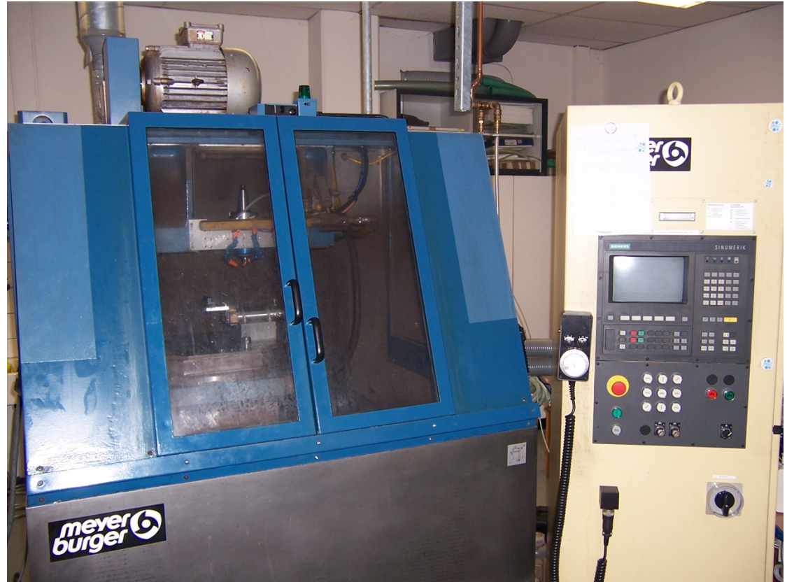
NC-controlled cutting with rotating blade or optional high speed milling tool, max thickness of work piece of 4 inch
