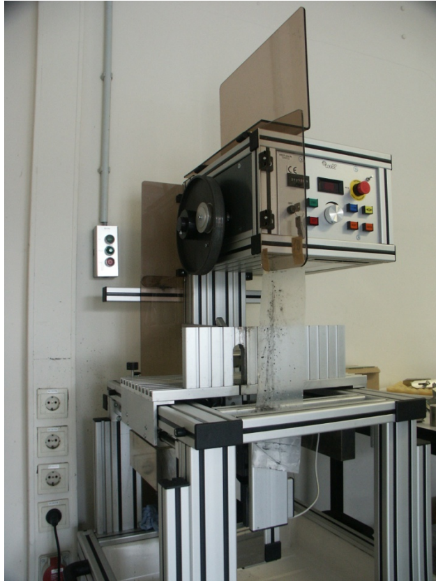
Wire-saw for coarse cutting of large Si pieces and special (hard) materials, i.e. tungsten, molybdenum
