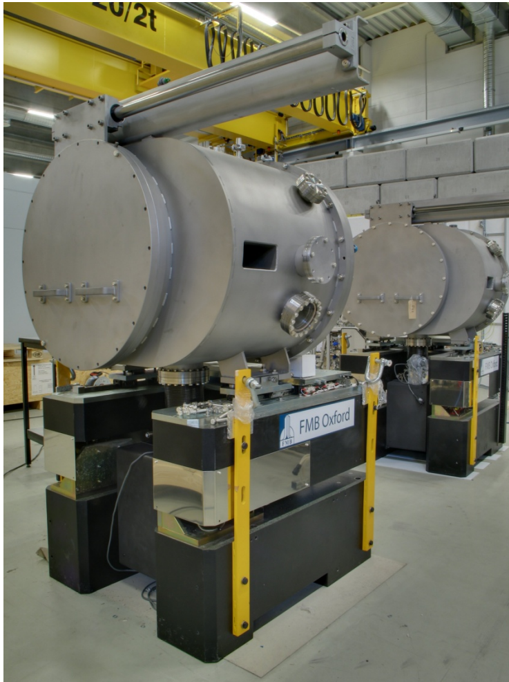
Monochromator systems for canted undulator sectors at PETRA III
