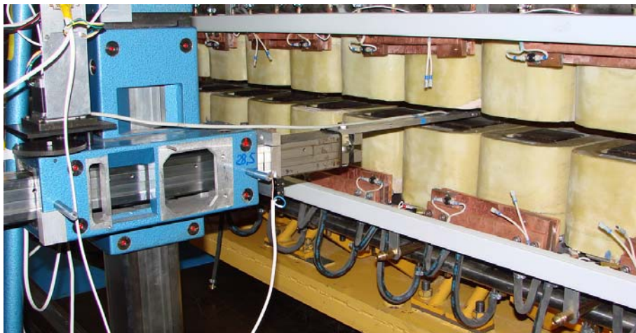
Figure 9 Measurement arm with Hall probe
