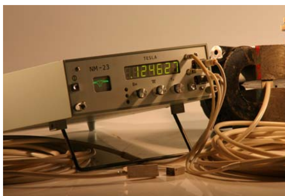
Figure 12 NM-23 NMR magnetometer
