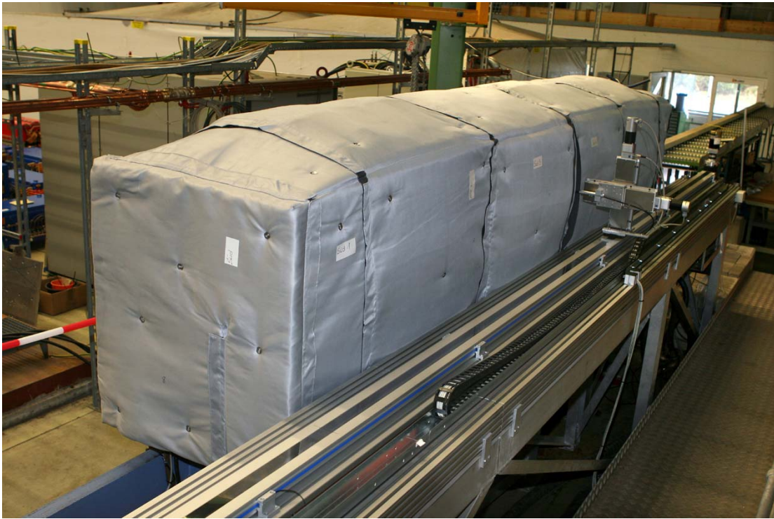
Figure 23 Undulator with thermal shield installed and Hall sensor inserted
