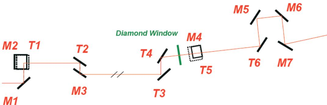
Figure 5: Optical layout of the IR undulator beamline (top view). Six toroidal mirrors and 7 planar mirrors are used to transport the IR radiation to the end of VUV beamline BL3 in the experimental hall.
