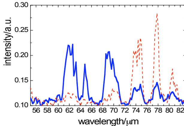
Figure 9: Spectra of the undulator radiation with the undulator tuned to nominal 60  $\mu\text{m}$  (blue solid) and to 70  $\mu\text{m}$  (red dashed). Clearly a red shift of the fundamental is observed in both cases. The spectra are modified by strong water absorption bands due to humidity in the laboratory air.
