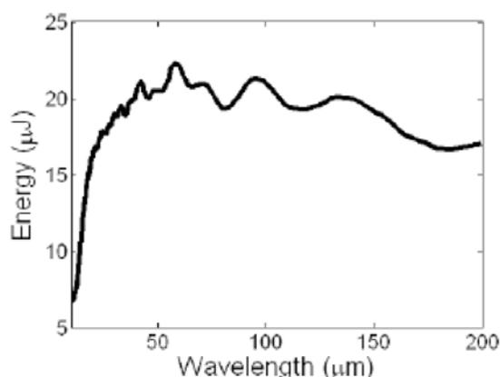
Figure 1: Pulse energies emitted into the central cone of the undulator considering the electron bunch form from reference [4] and a contributing bunch charge of 1 nC (courtesy of O. Grimm and M. Yurkov).
