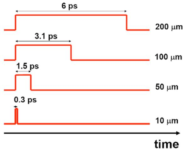
Figure 2: IR pulses emitted from the IR undulator tuned to a wavelength of 200, 100, 50 and 10  $\mu\text{m}$ .
