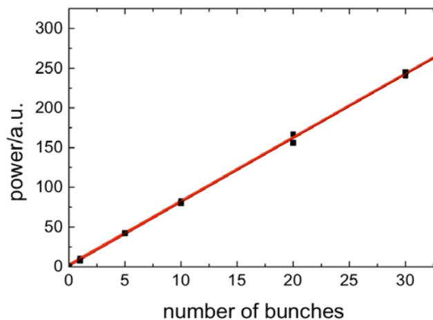
Figure 8: Dependence of the measured power on the number of bunches in one bunch-train. The bunch-trains are delivered with a repetition rate of  $5\ \text{Hz}$ . Measurements were taken through a band pass filter system with a center wavelength of  $100\ \mu\text{m}$ . The undulator was tuned to nominal  $85\ \mu\text{m}$ .
