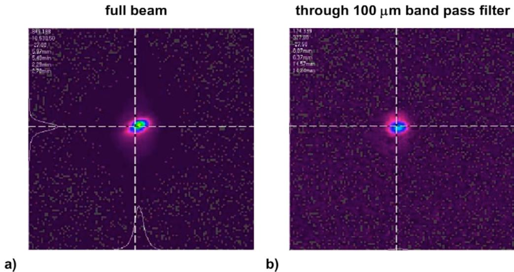
Figure 7: Beamprofile on a SPIRICON IR camera of the full beam (a) and through a band pass filter system with a center wavelength of  $100\ \mu\text{m}$  (b). The undulator was tuned to nominal  $85\ \mu\text{m}$ . The slightly elliptical shape is due to a misalignment of the outcoupling off-axis parabolic mirror in front of the provisional experimental station.
