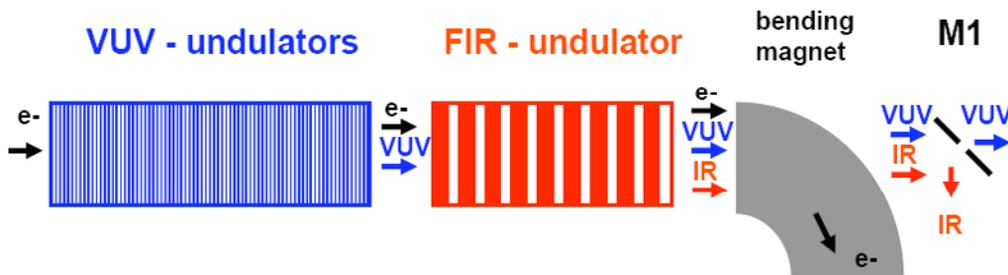
Figure 3: Arrangement of the FIR and VUV undulators in the FLASH accelerator tunnel. The FIR undulator uses the spent electron beam from the VUV undulators. The emitted IR pulse is thereby naturally synchronized to the VUV pulse. The IR beam is coupled out by the first mirror M1 of the IR beamline.
