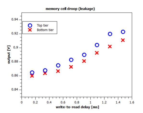
significant parasitic leakage of charge stored in memory cells
