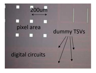
10x test structure for TSV evaluation: daisy chain of 64 TSVs, by connected M1/backM.
