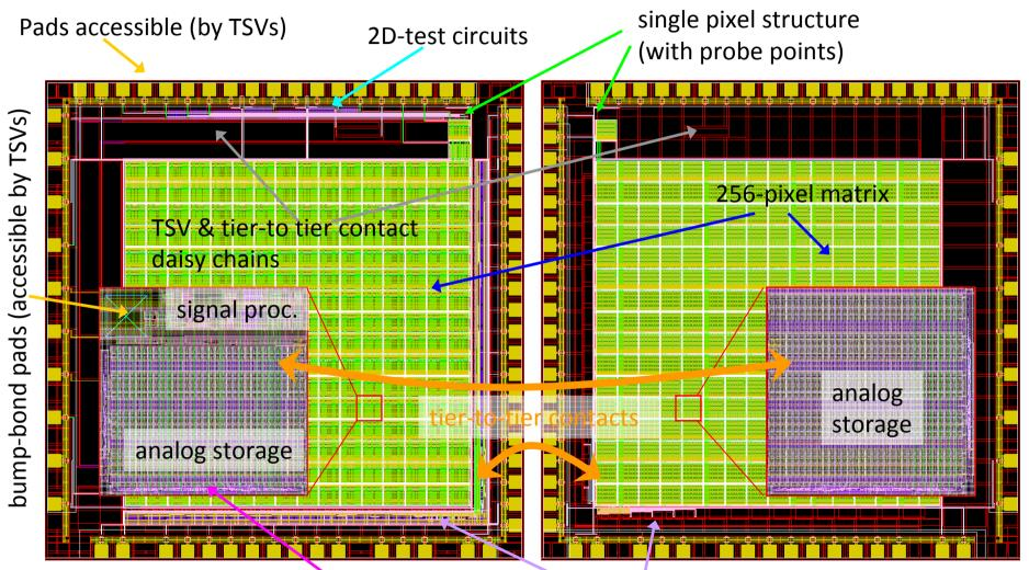
SC-based addressing circuit (distributed on both tiers) both at the pixel level and at the array level
