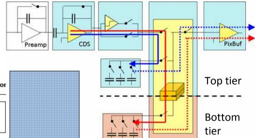
expected operation region of the circuit: comparable (linear) behaviour of the detector output, whether the charge is stored in/read from storage cells located on the Top tier or Bottom tier
