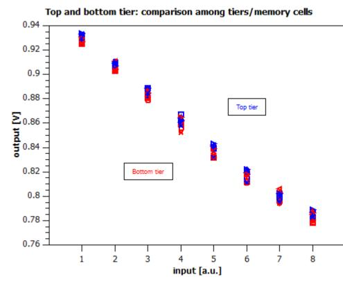
Comparable (linear) detector response - for charge stored in either in Top/Bottom tier - for different memory cells in the same pixel, independently from their location. Slight pedestal offset, to be investigated further
