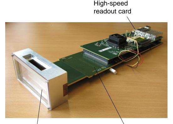
Detector head with Si sensor
