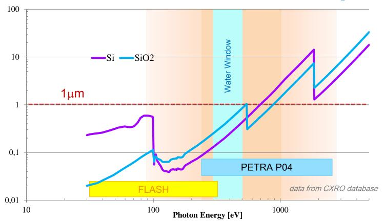
At (very) soft X-ray energies, QE is limited by passive window thickness!
