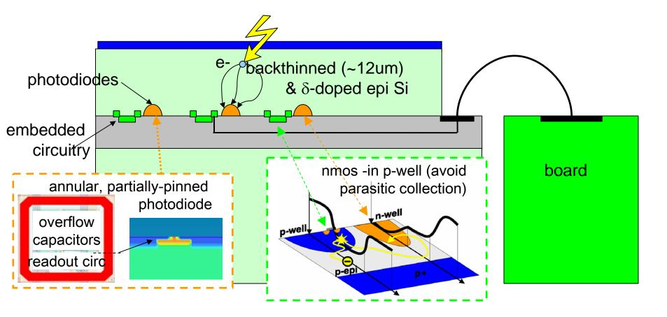
Monolithic: Collecting diodes & readout circuitry share the same substrate TowerJazz 0.18um CMOS techn, over high-resistance thick epi Coupled to handling wafer, back-thinned, back-illuminated: 100% fill factor Back surface delta-doped, post-processed: almost no entrance window
