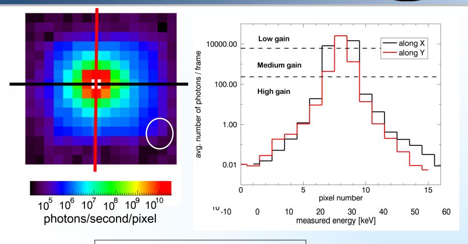
Gain switching experimentally proven ➤ 10<sup>4</sup> photons / pulse ➤ Single photon sensitivity ➤ 4.5 MHz frame rate
