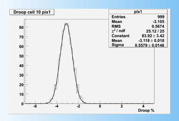
Droop distribution over 1000 frames for 1 cell ( cell #10) in pixel 1.
