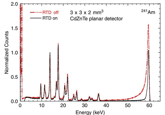
Fig. 5. Two  $^{241}\text{Am}$  spectra taken with a  $3 \times 3 \times 2 \text{mm}^3$  CdZnTe detector, illustrating the effectiveness of risetime discrimination. From the figure, we see that the hole tailing is substantially reduced when RTD is used and in fact the FWHM energy resolution improves from  $\sim 1$  keV to 700 eV at 59.54 keV. However, an energy-dependent decrease in photopeak efficiency is also apparent.
