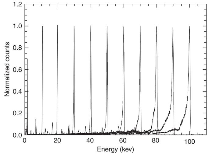
Fig. 2. Composite pulse height spectra of monoenergetic lines measured at HASYLAB. The beam size was  $20 \times 20 \mu\text{m}^2$ , incident at the center of the detector.
