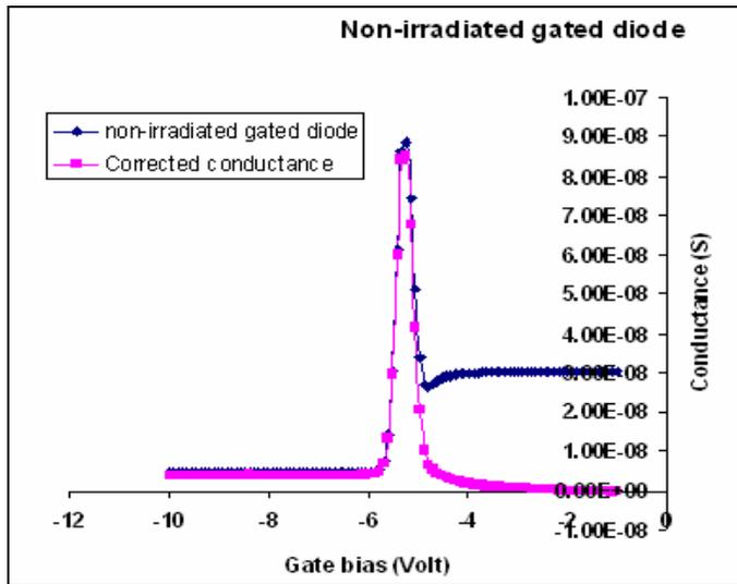
Figure 4a: Corrected conductance as function of gate bias at for non-irradiated gated diode at 10 kHz.
