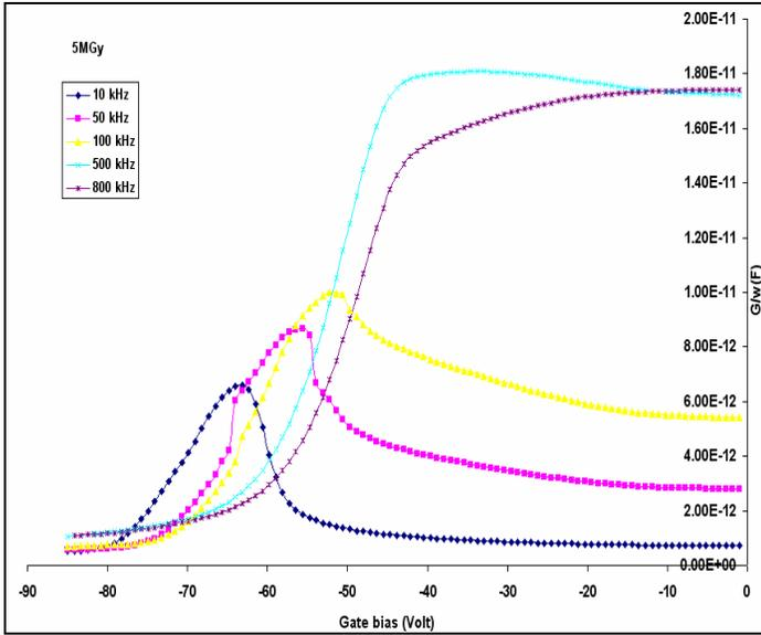
Figure 6a: Conductance ( $G/\omega$ ) at different frequency as a function of gate bias for 5 MGy irradiated gated diode.
