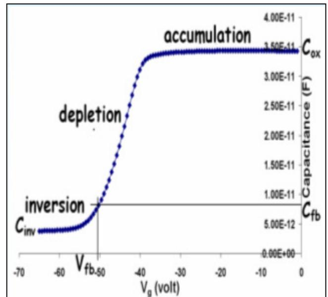
Figure 1 b: Typical Capacitance-Voltage ( $C/V_g$ ) curve. In Fig 1.1,  $C_{ox}$ - oxide capacitance [F],  $C_{inv}$ - HF inversion capacitance,  $V_{fb}$  – flat band voltage and  $C_{fb}$ - flatband capacitance.
