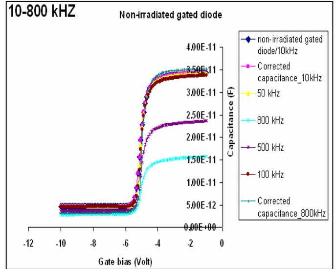
Figure 3a: C/V<sub>g</sub> as function of frequency for non-irradiated gated diode.
