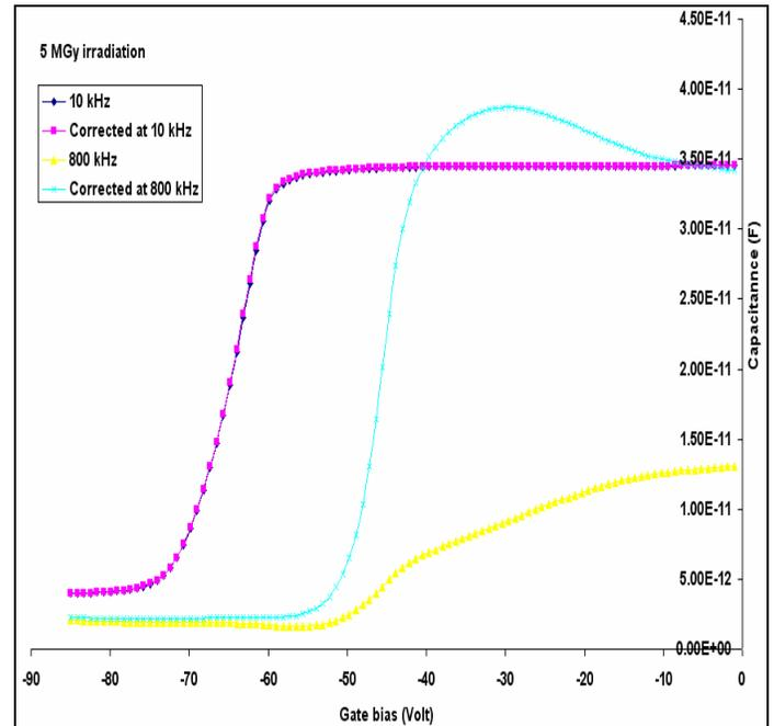
Figure 7: Corrected capacitance at 10 and 800 kHz as function of gate bias for 5 MGy irradiated gated diode.
