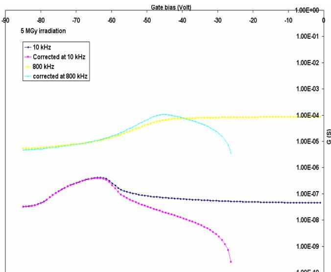
Figure 6b: Conductance ( $G$ ) at 10 and 800 kHz frequency as a function of gate bias for 5 MGy irradiated gated diode.
