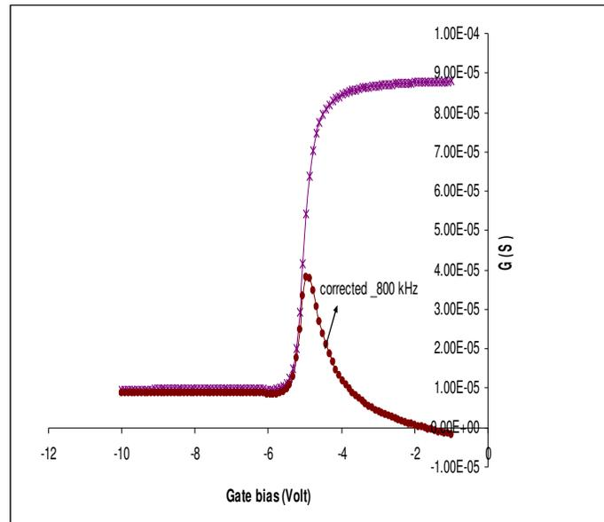
Figure 4b: Corrected conductance as function of gate bias at for non-irradiated gated diode at 800 kHz.
