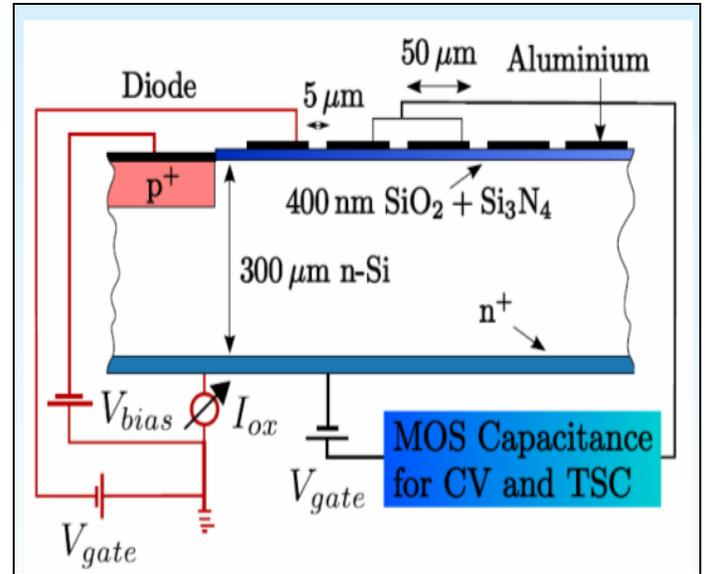
Figure 1a: Schematic of the gated diode (five gate rings) structure. Circuit for  $I/V_g$  and  $C/V_g$  measurements are shown in the left and right part of the structure (here the results are shown for the measurement performed immediately after irradiation).
