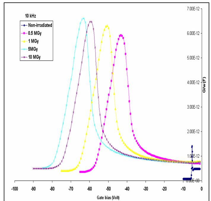
Figure 5: conductance ( $G/\omega$ ) as function of gate bias at for different irradiated gated diode at 10 kHz.
