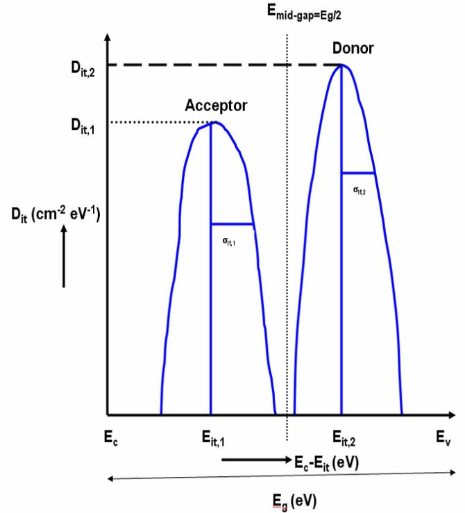
Figure.2: Two Gaussian distribution of interface trap model for TCAD simulation of surface damage effect in Si sensors.
