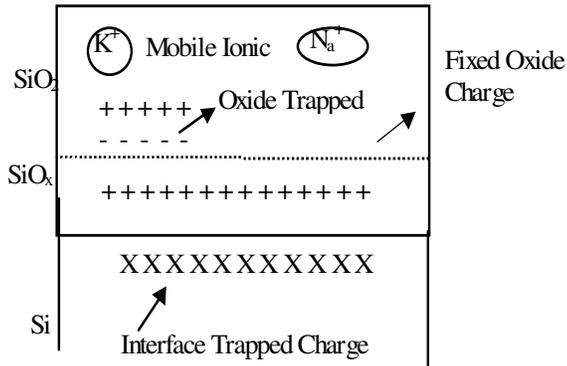
Figure 1c : Charges and their location for thermally oxidized silicon.
