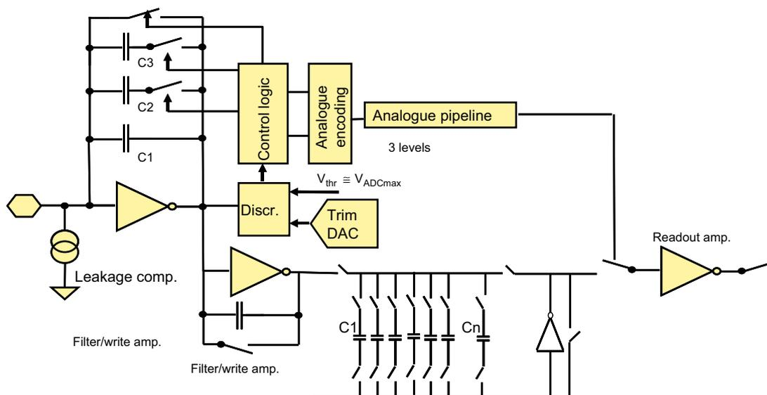
Fig. 1. Schematic of the proposed pixel cell.
