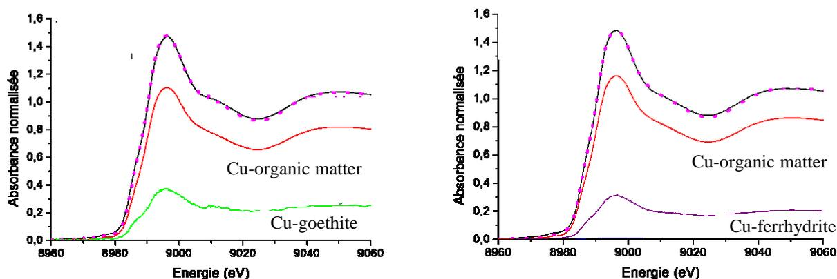
Figure 1: Example of experimental XANES spectra and the linear combination fitting results.
