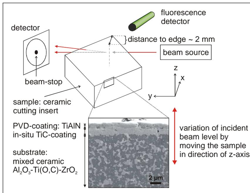
Figure 1: Schematic display of the experimental set-up.
