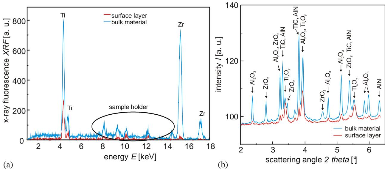
Figure 2: Fluorescence spectra (a) and diffraction patterns (b) of the bulk and the coating of a mixed ceramic cutting tool material.
